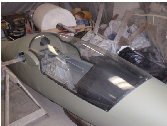
Prime prior to paint
